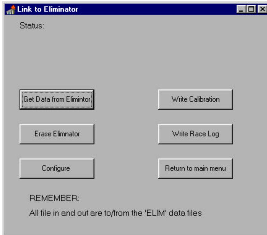
1. Depress the Get Data from Eliminator button to download the information from the Eliminator. You must make sure that the Eliminator 2000 is in the PC Linkup mode. Refer to the Snap-In<sup>™</sup> Weather Manual for Linkup information.
